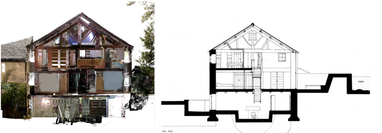
Figure 17. The juxtaposition of the cross-section post-produced after scanning (left) (Image by authors); The original design cross-section (right) (Image by Peter Blundell Jones)
